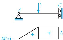
$$\downarrow \Delta_B = \int \frac{M\bar{M}}{EI} dx = \frac{1}{EI} \times \left[ \frac{(P-F)L \times L \times L}{3} + (P-F)L \times L \times L \right] = \frac{4(P-F)L^3}{3EI}$$
